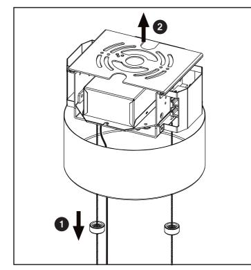
**Step 1** Loosen the bolt on the canopy.
