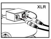
Connect DMX by using a standard shielded
