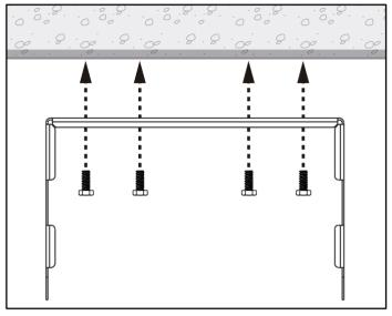
Step 4 Fasten the top bracket on the desired location on the ceiling.
