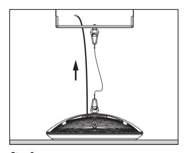
Step 3 Attach the fixture cables through the lower bracket.
